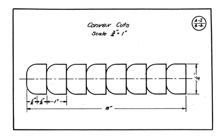
The class project is turned from kiln dried construction grade 2x4 to show how inexpensive or free wood may be used for practicing basic tool handling and control.
